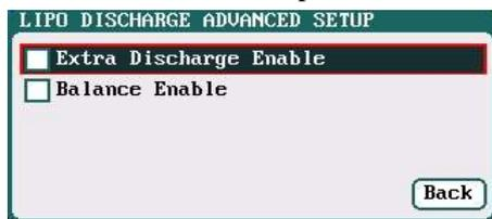
➤Note: 1. Tick *Extra Discharge Enable* to activate *discharge enable*, see more details on [“Lithium Battery Extra Discharge Mode”](#).
