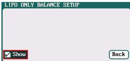
➤ *Note: Balance Only is the program only to equalize the individual cells through balance port to reduce the voltage difference.*
